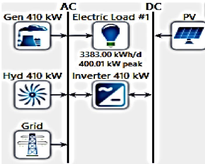
Fig. 4 Owena Small hydropower-solar PV-diesel generator model
