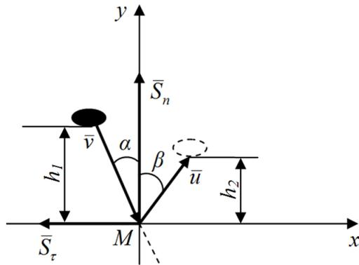
**Fig. 5.** Scheme for studying the collision of onion seeds with soil
