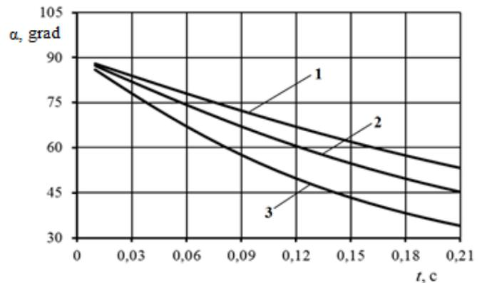
**Fig. 8.** Graphic dependences of the angle of incidence of onion seeds during the fall
