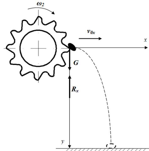
**Fig. 2.** The scheme for determining the trajectories of onion seeds during the release
