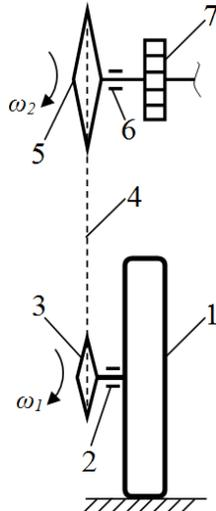
1-wheel support, 2, 6-bearing, 3-wheel sprocket; 4-flail; 5-driven sprocket; 7-disc meter
