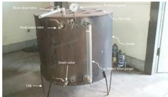
Picture 1. Fire Pipe Boilers
