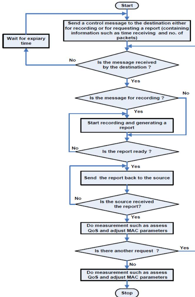
**Figure 7:** Proposed method for measuring the QoS parameters and adjusting MAC protocol transmission parameters such as CWmin value in physical networks.
