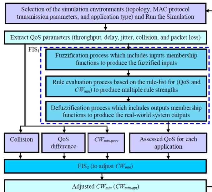
Figure 3: Fuzzy logic model for assessing QoS and optimising the CWmin value.
