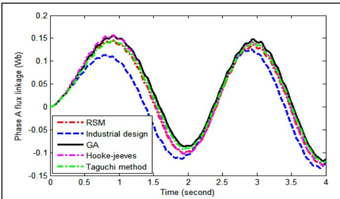
Fig. 4. Phase A flux linkage characteristics at 21,000 rpm
