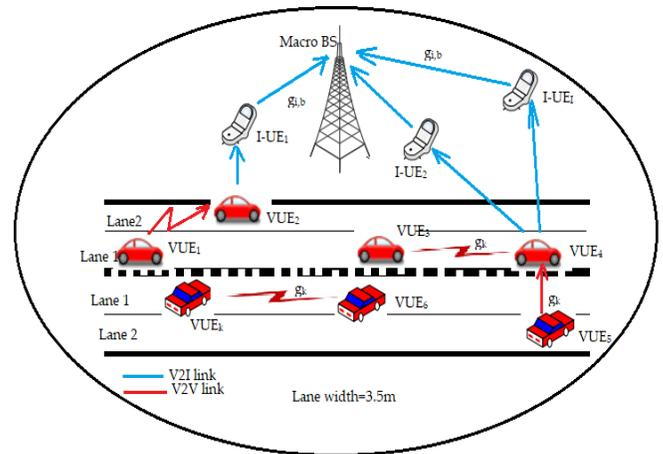
Figure 1: D2D-enabled vehicular network model
