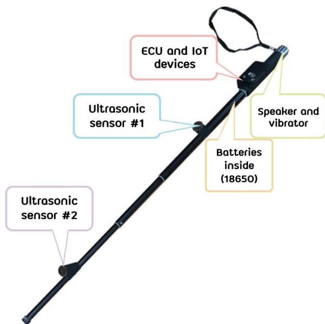
**Fig. 3.** The walking stick with IoT and sensor devices for blind people.
