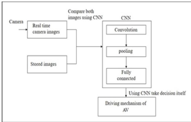
**Fig. 1** Schematic of CNN for an autonomous vehicle
