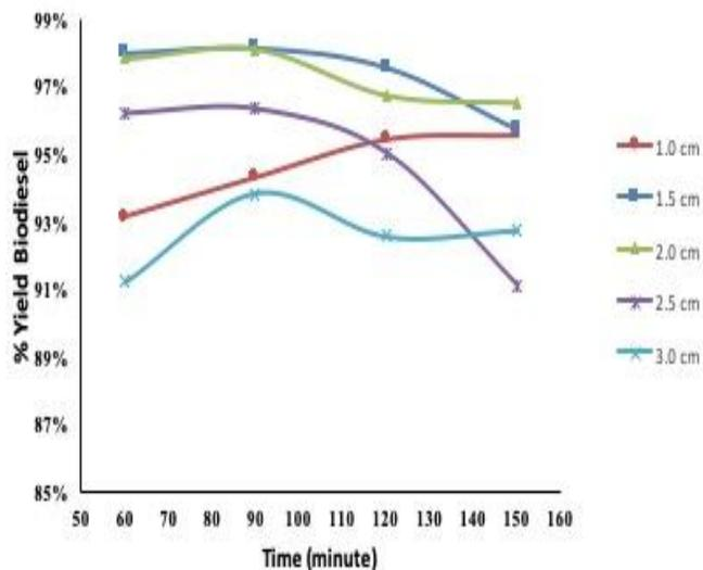
Fig. 6 Impact of time of process to yield of biodiesel
