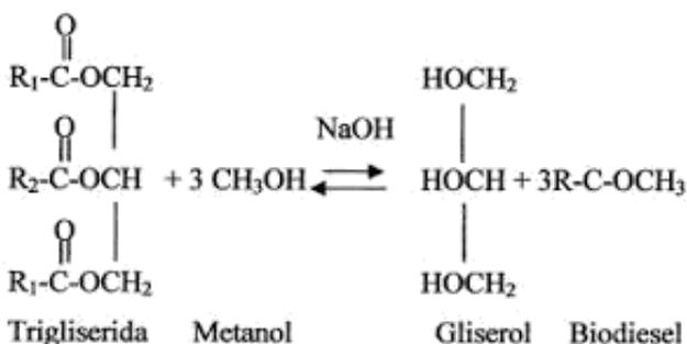
Fig.1. Transesterificate reaction
