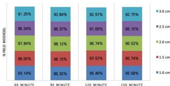
Fig. 5. Biodiesel yield on electrode space variation and time of reaction
