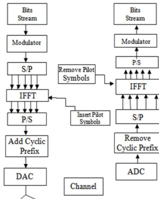
Fig.2 Block Diagram of OFDM Communication [2]
