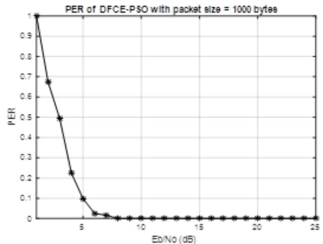
**Fig. 5:** PER of proposed DFCE with packet size = 1000 bytes in 140 km/h mobility
