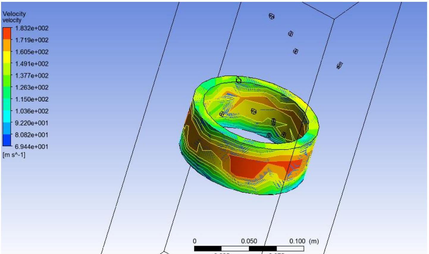
**Fig 9** VELOCITY OF POLYMER MEDIA
