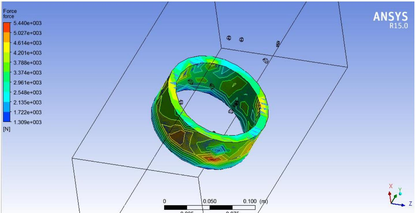
**FIG.8** FORCE APPLIED ON POLYMER MEDIA ON WORKPIECE
