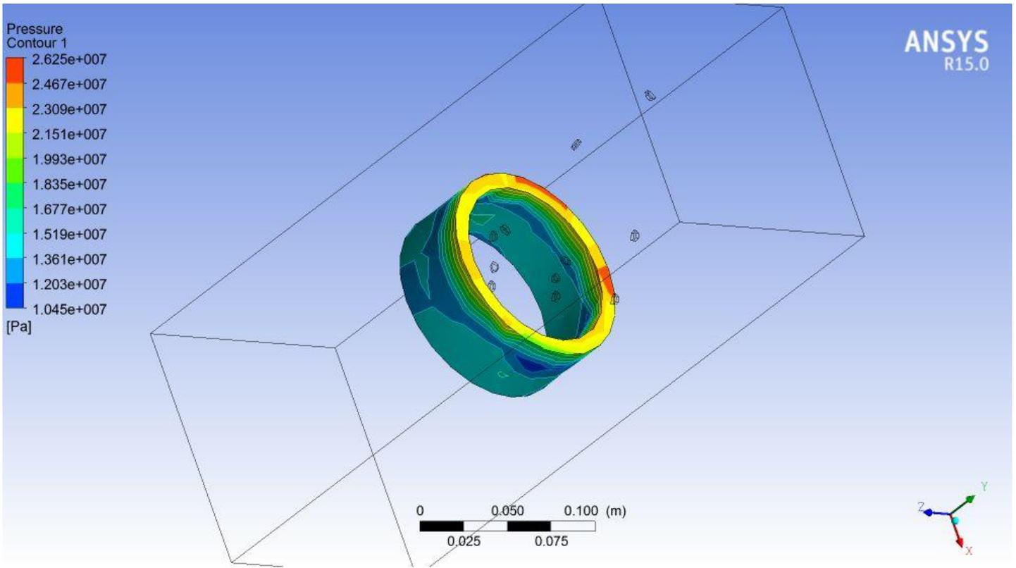
**FIG.6 EFFECT OF PRESSURE VARIATION ON WORKPIECE**
