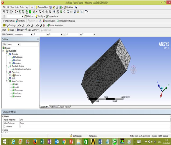
Fig. 2. Meshing of Fluid Domain
