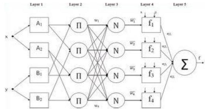
Fig. 1. The ANFIS structure that has two inputs and one output
