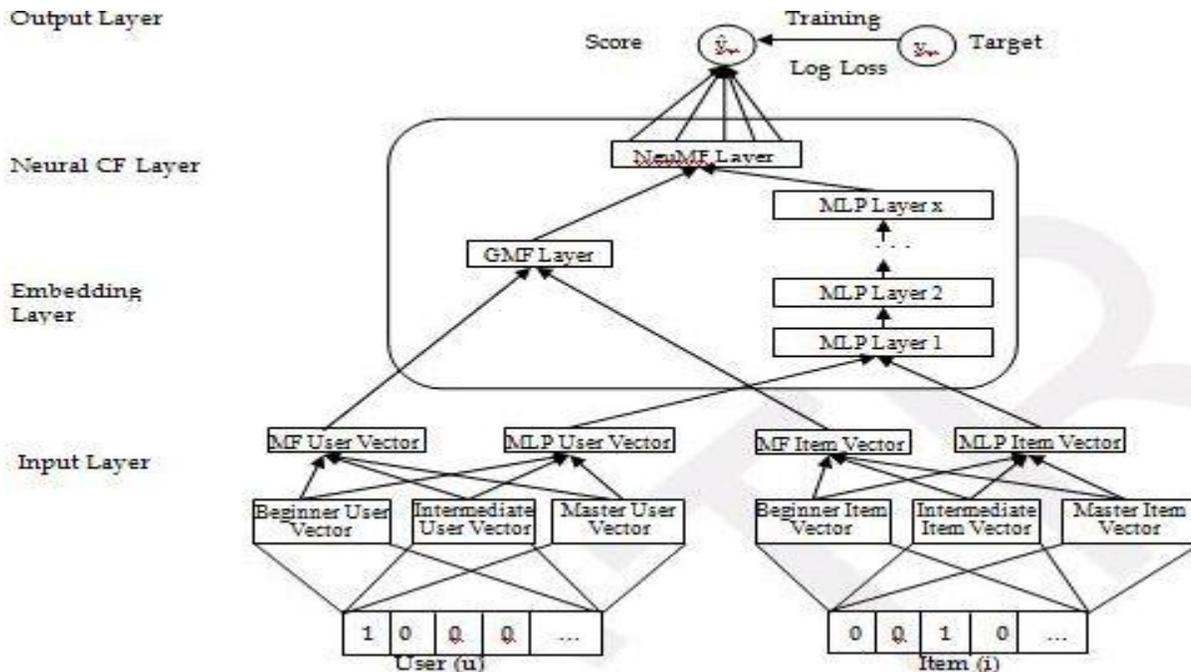
Fig.2. Group Based Neural collaborative Filtering
