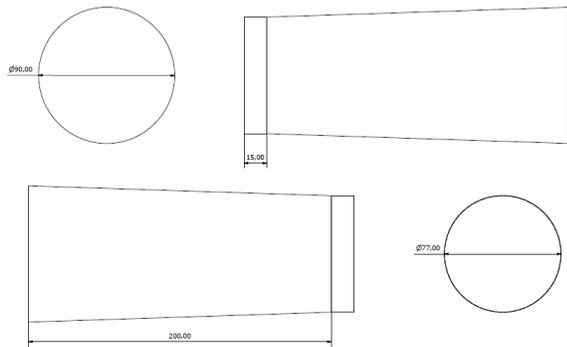
**Fig. 4.** The Engineering Drawing of Rasayana Racing Plane Inlet
