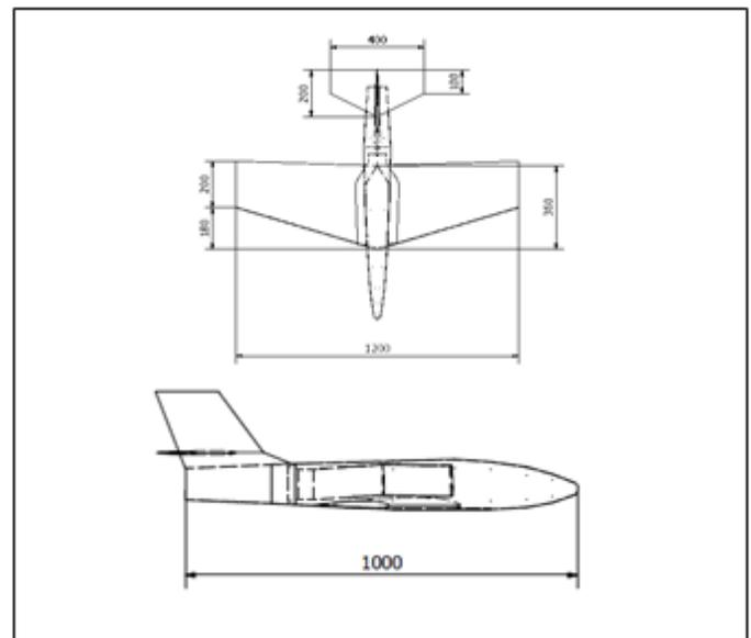
Fig. 2. The Engineering Drawing of Rasayana Racing Plane
