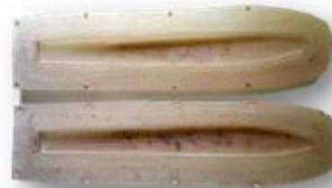
**Fig. 7.** Negative Mold of UAV Fuselage.
