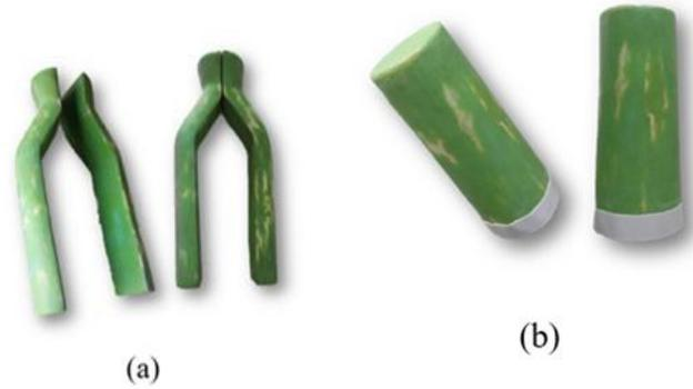
**Fig. 6.** Positive Mold of Air Duct (a) Inlet Tube (b) Outlet Tube
