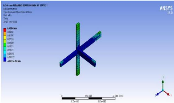
Fig.15. Equivalent stresses developed in structure with 378 mm anchorage
