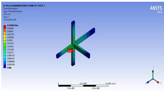
Fig. 9. Deformation of structure with 10d=160 mm anchorage
