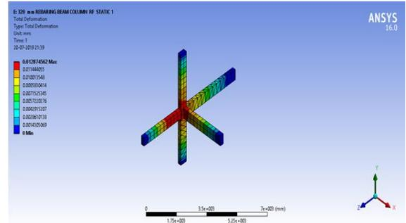
Fig. 11. Deformation of structure with 20d=320 mm anchorage
