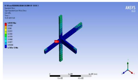
Fig. 14. Equivalent stresses developed in structure with 378 mm anchorage
