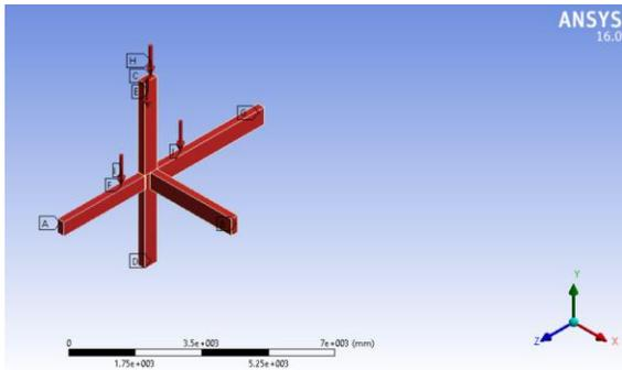
Fig. 7. Post-installed connection with boundary conditions
