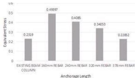
Fig.16. Anchorage length V/S Stress
