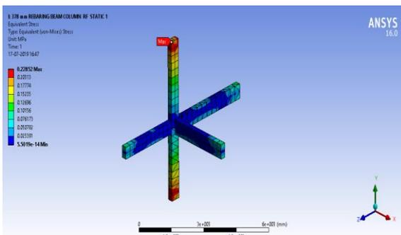
Fig.17. Equivalent stresses developed in structure with 378 mm anchorage
