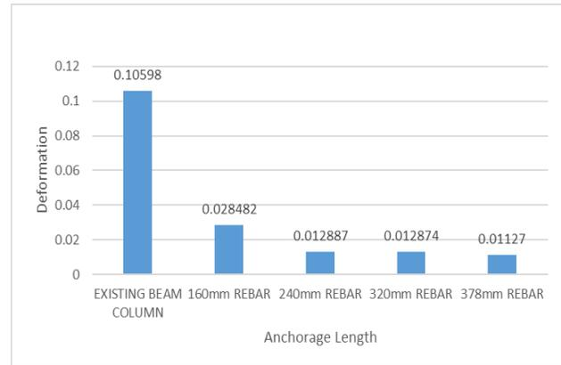
Fig.15. Anchorage length V/S Deformation
