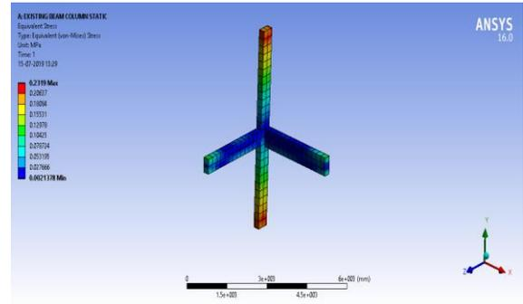
Fig. 13. Equivalent stresses developed in structure with 378 mm anchorage
