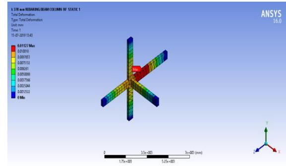
Fig. 12. Deformation of structure with 378 mm anchorage
