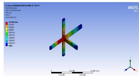
Fig. 10. Deformation of structure with 15d=240 mm anchorage
