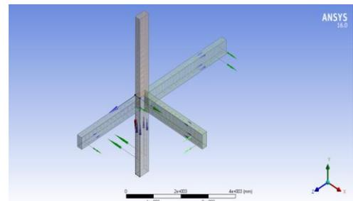
**Fig. 5.** Geometry of post-installed connection to existing structure
