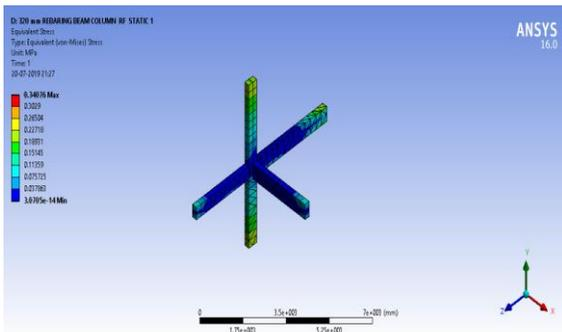
Fig.16. Equivalent stresses developed in structure with 378 mm anchorage
