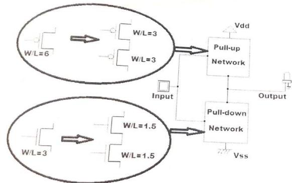
Figure 5 : Stack transistor
