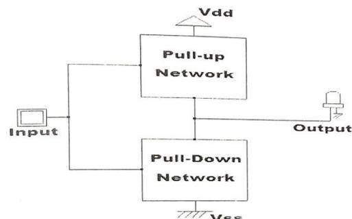
Figure 1 - Conventional CMOS inverter
