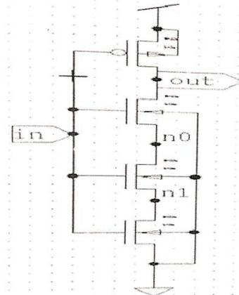
Figure 4: Forced 2 NMOS transistor
