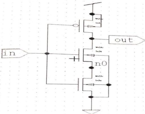
Figure 2 – Forced NMOS transistor
