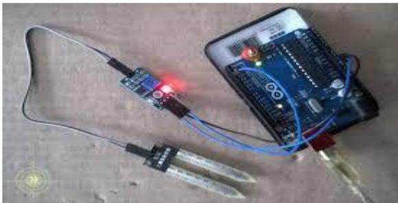
Fig. 3. Soil moisture sensor with Arduino board
