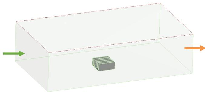
**Figure 2:** Boundary conditions for forced convection case.
