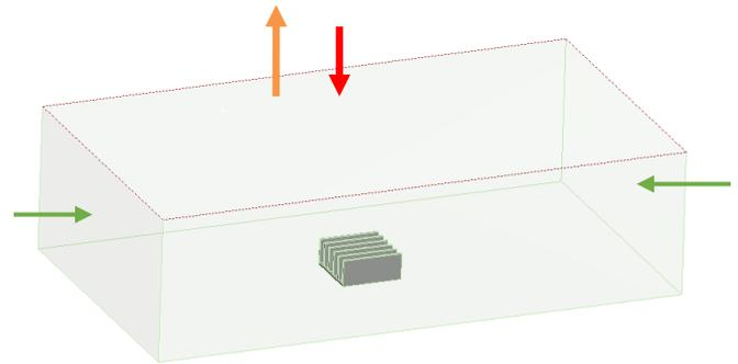
**Figure 3:** Boundary conditions for natural convection cases.
