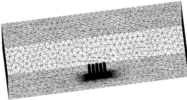
Figure 4: Mesh model of the heat sink with fluid domain
