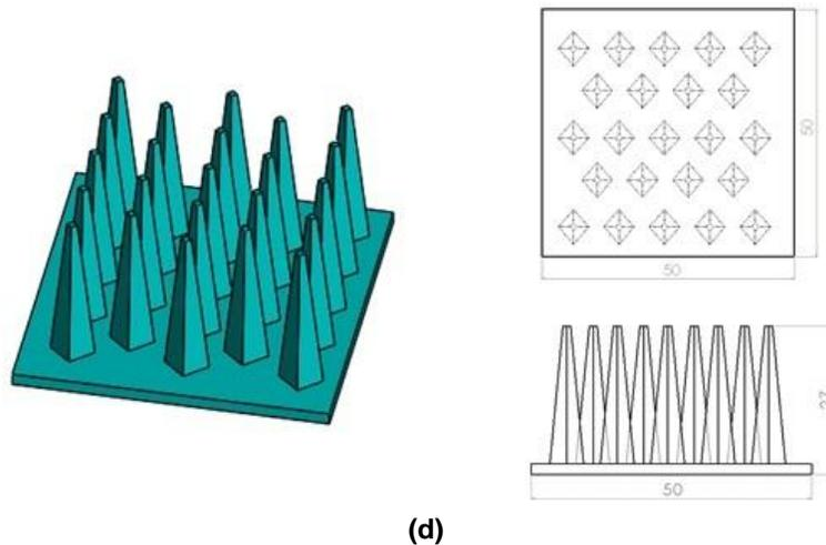
**Figure 1 (a, b, c, d):** Three views namely iso, top, front represented in the above figures for inline and staggered heat sink with Rhombus prism pin fin and also heat sink with Rhombus pyramid pin fin.
