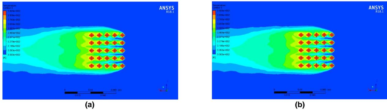
Figure 8 (a), (b): Rhombus pyramid with inline pins – (Al, Cu)
