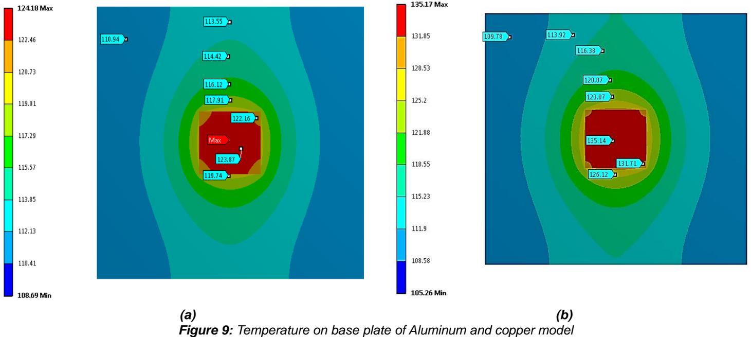
Figure 9: Temperature on base plate of Aluminum and copper model
