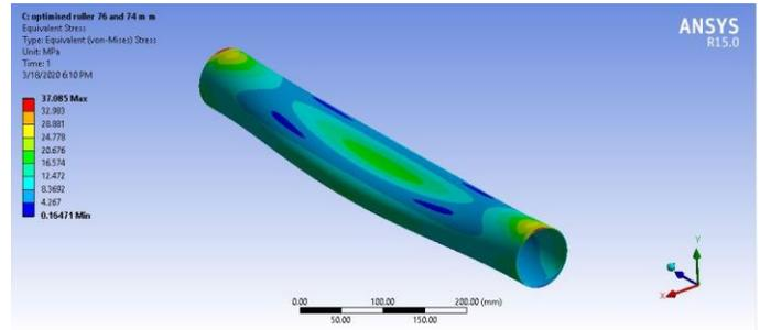
**Fig. 5. Equivalent Stresses in Optimized Roller**
