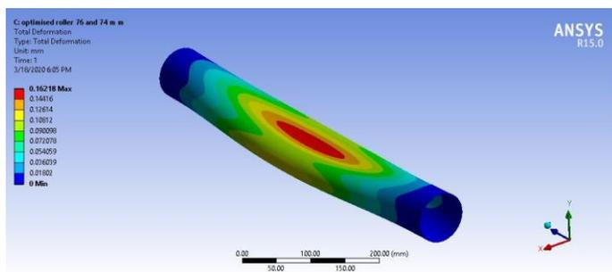
**Fig. 4. Total Deformation of Optimized Roller**
