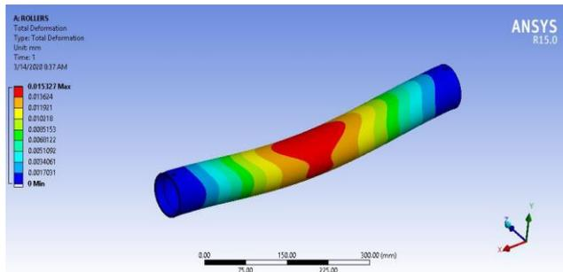
Fig. 2. Total Deformation of Existing Roller
