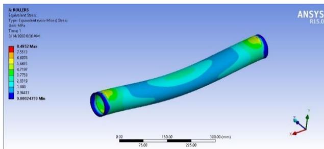
Fig. 3. Equivalent Stress in Existing Roller.
