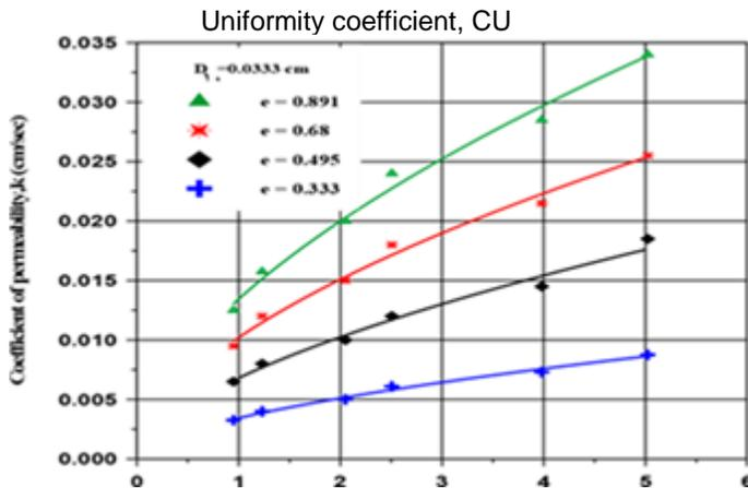
Figure 4: relationship between (K),(CU)and(e) for site (A)
