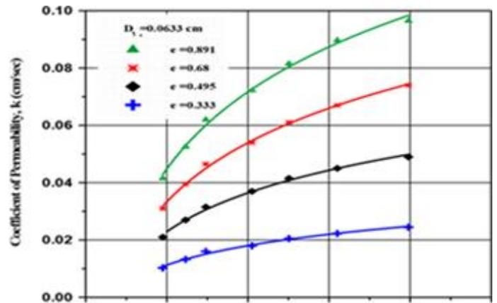
Figure 5: relationship between (K),(CU)and(e) for site (B)
