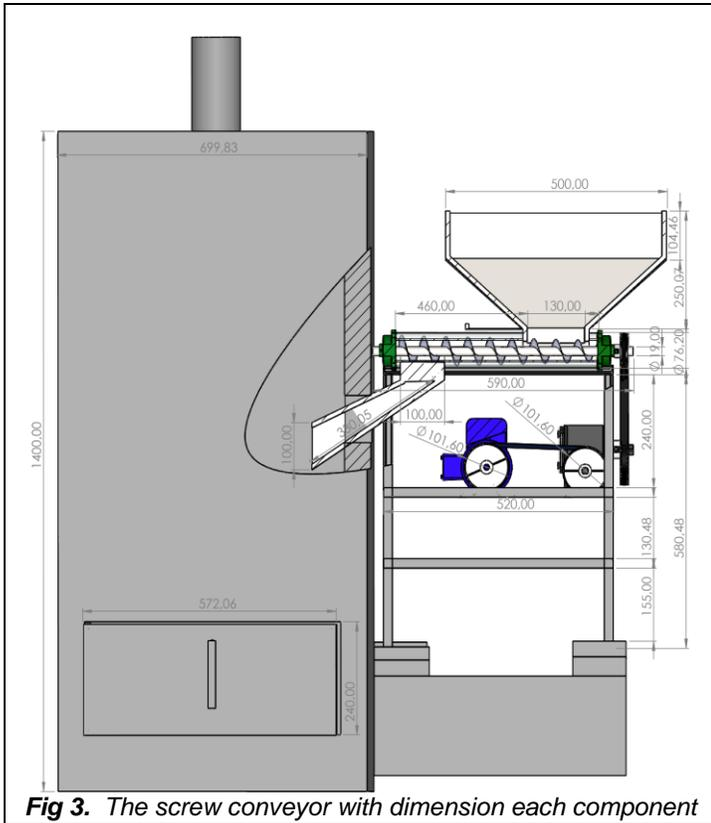
Fig 3. The screw conveyor with dimension each component
