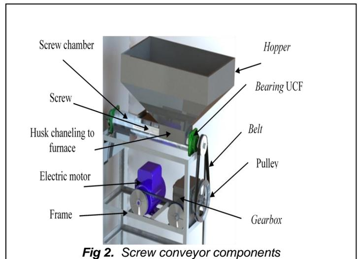
**Fig 2.** Screw conveyor components
