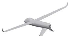
**Fig. 3.** Aircraft with low (V-Inverted tail) configuration
