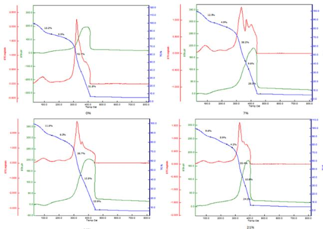
**Figure 2. Results of Thermal degradation on TBP Treated Leathers**
