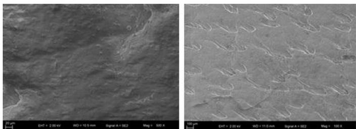
**Figure 5.** SEM image of 7% Leather Samples in 20  $\mu\text{m}$  and 100  $\mu\text{m}$  Magnification
