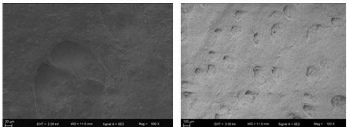
**Figure 6.** SEM image of 14% Leather Samples in 20  $\mu\text{m}$  and 100  $\mu\text{m}$  Magnification
