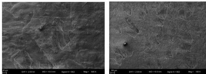
**Figure 7.** SEM image of 21 % Leather Samples in 20  $\mu\text{m}$  and 100  $\mu\text{m}$  Magnification
