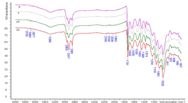
**Figure 3. ATR-FTIR Spectra of TBP Treated Finished Leathers**
