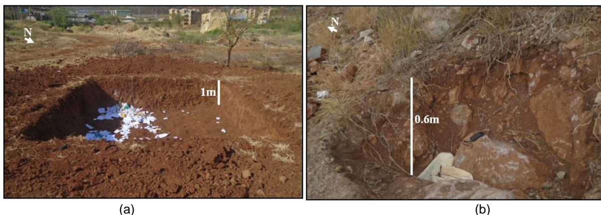
Figure 2.1. (a) A dump pit which was used for sampling soil from the reddish- brown soil unit. (b) An abandoned construction pit on the vesicular basalt unit which is used for rebound hammer testing.
