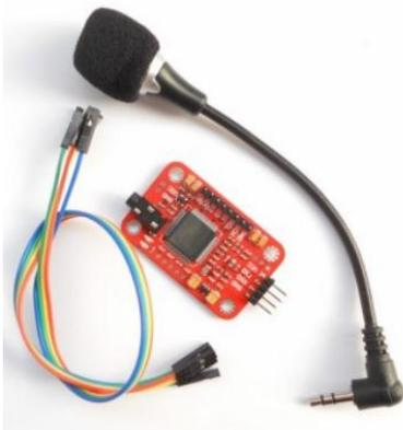
**Figure 7. Pictorial view of VR3 voice recognition module.**
