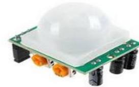
Figure 5. Pictorial view of PIR module
