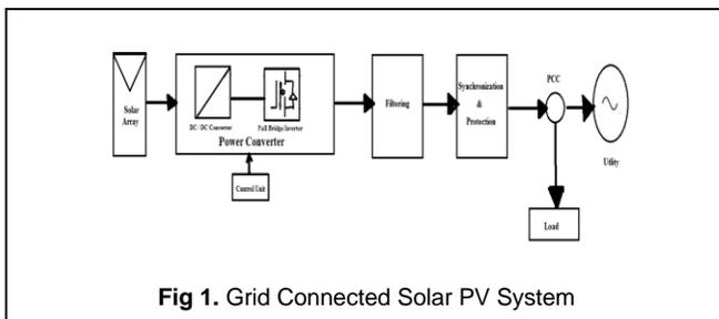
The grid connected solar PV system is composed of solar PV array, boost converter, power inverter and utility grid as shown in Fig. 1. Solar PV array generates DC power at its maximum using boost converter with MPPT algorithm whereas power inverter converts this DC power to AC power and feeds to utility grid.
