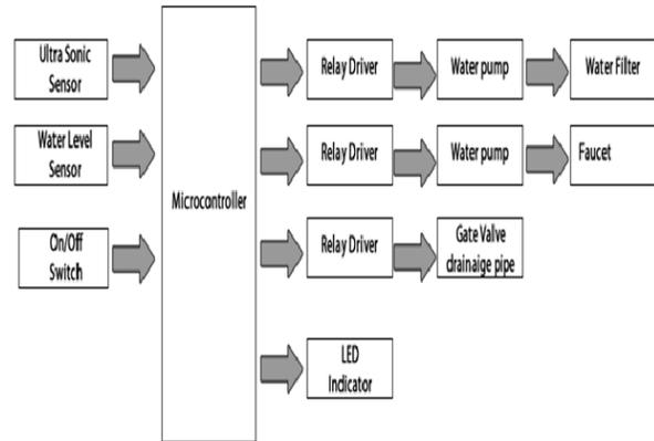
**Fig. 3** Block Diagram of the Wastewater Management System.
