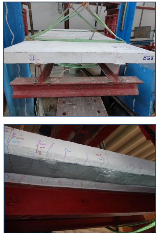
FIG.(9) Crack Patterns at Failure for BG8
