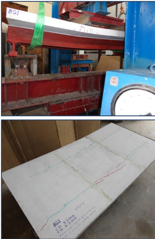
FIG.(6) Crack Patterns at Failure for BG1-Control Sample
