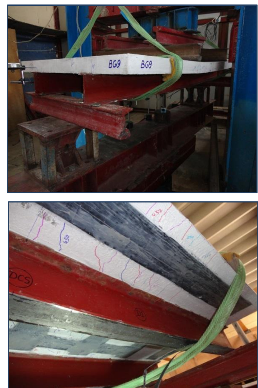
FIG.(10) Crack Patterns at Failure for BG9
