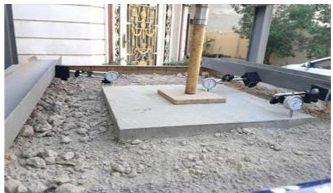
Fig. 2 Concrete slab during the test
