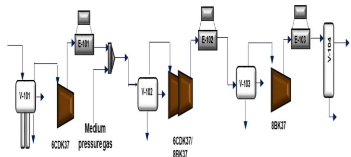
Fig. 1. Compressor train arrangement.
