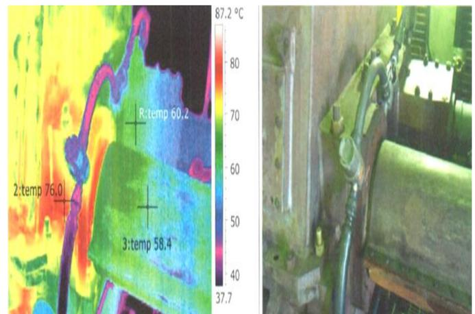
**Fig. 5.** Main gear thermographic image (turbine side).
