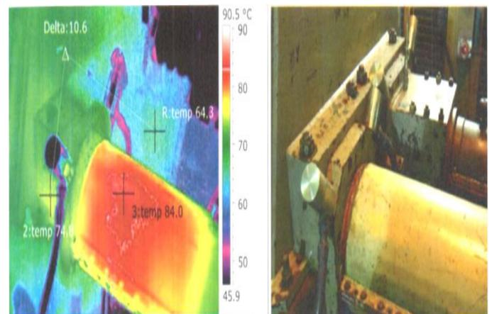
**Fig. 6.** Main gear thermographic image (compressor coupling side).
