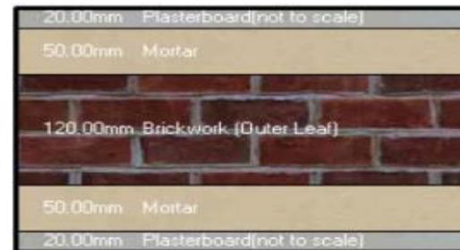
**Figure 1** Represents Section of the Existing Wall Layers
