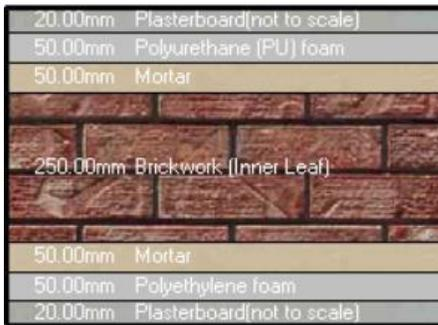
**Figure 2** Represents Section of the optimized wall Table 4 Represents all Layers for the Optimized Walls:-
