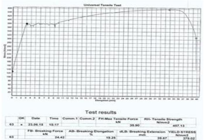
Fig. 3. Test Result of the Tensile Test on 10mm High Yield Steel Bar.
