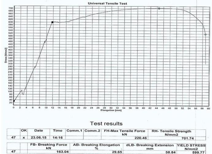
Fig. 12. 25mm Mild Steel Tensile Strength Test Result.
