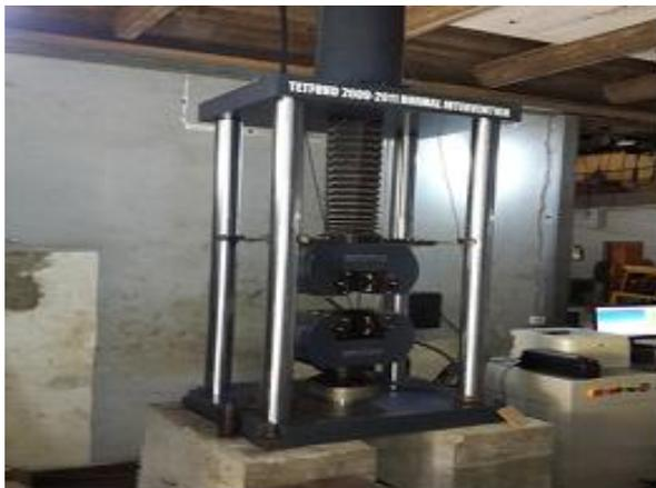
Fig. 2. Hydraulic Universal Test Machine
