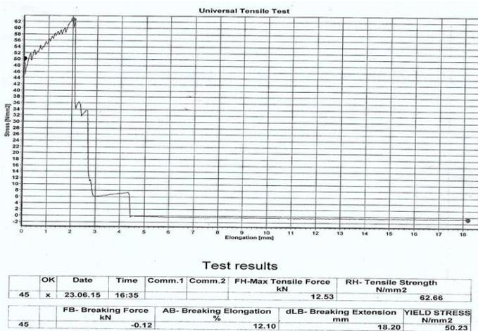
Fig. 16. 20mm Bamboo Tensile Strength Test Result.
