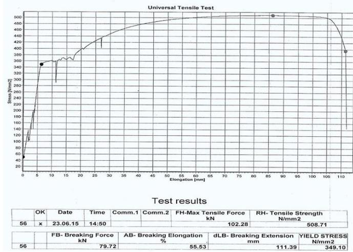
Fig. 10. 16mm Mild Steel Tensile Strength Test Result.
