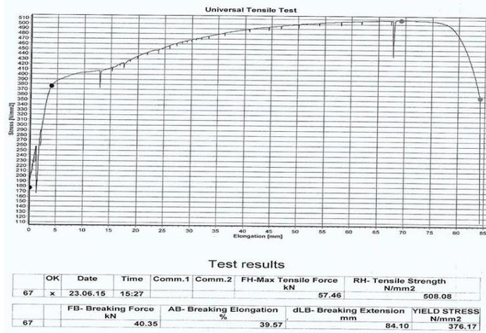
Fig. 9. Tensile Strength Test Result for 12mm Mild Steel.
