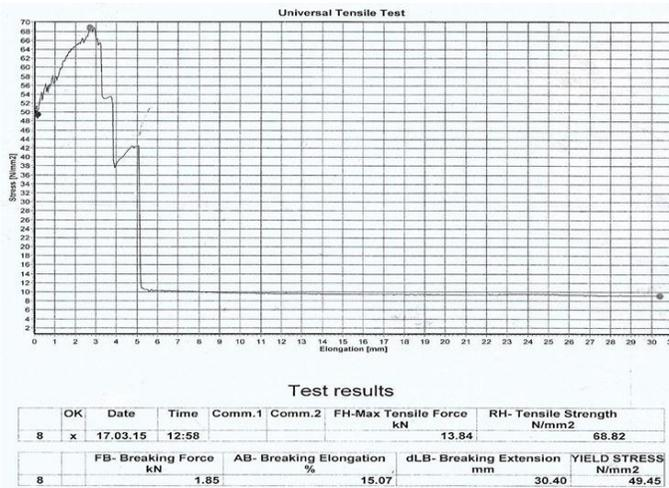
Fig. 15. 16mm Bamboo Tensile Strength Test Result.
