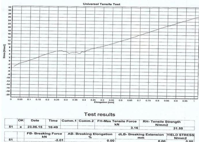
Fig. 13. 10mm Bamboo Tensile Strength Test Result.
