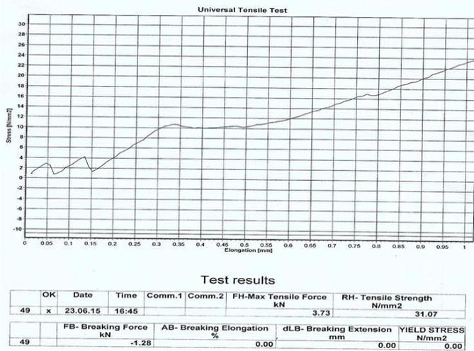
Fig. 14. 12mm Bamboo Tensile Strength Test Result.
