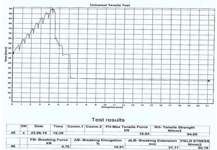
Fig. 17. 25mm Bamboo Tensile Strength Test Result.
