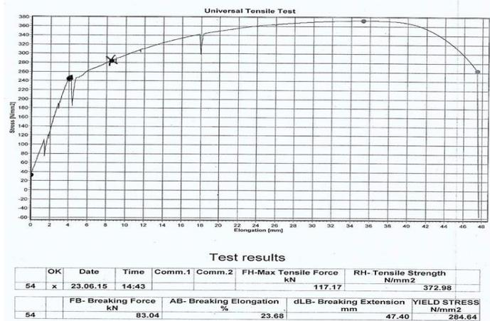
Fig. 11. 20mm Mild Steel Tensile Strength Test Result.
