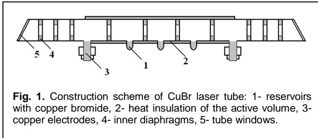
Fig. 1. Construction scheme of CuBr laser tube: 1- reservoirs with copper bromide, 2- heat insulation of the active volume, 3- copper electrodes, 4- inner diaphragms, 5- tube windows.
