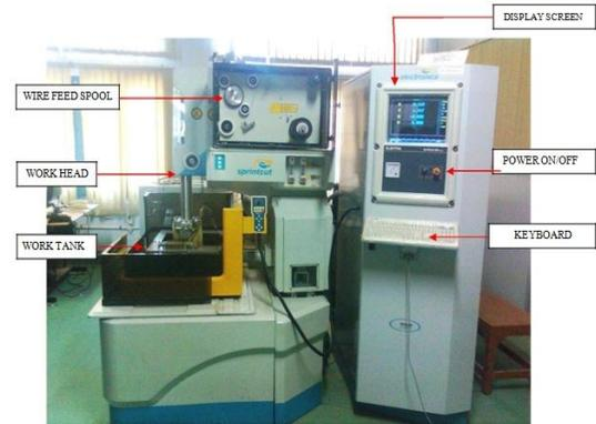
**Figure 2:** Pictorial View of WEDM Machine Tool
