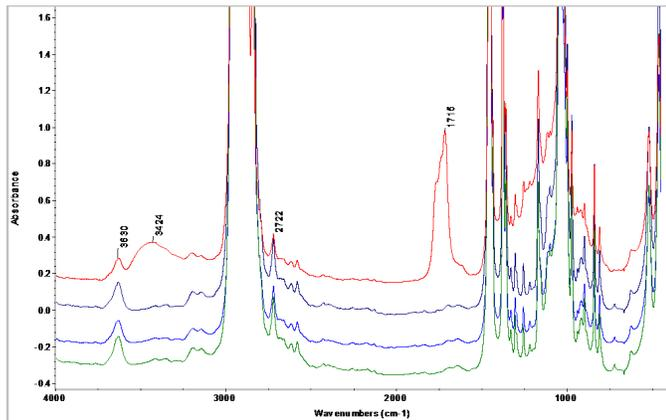
**Figure 2.3.** The results of FTIR analysis of nanocomposite PP / MMT-Clay without antioxidants
