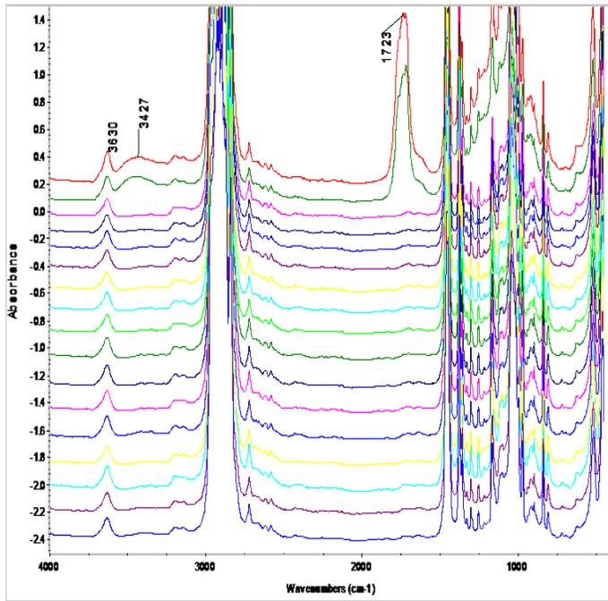
**Figure 2.1.** The results of FTIR analysis of nanocomposite PP / MMT-Clay-Irganox 1010 after warmer at a temperature of 180°C for 10 min and expose to Wallace Oven on 0-518 hours.
