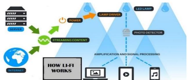
Figure 2. Construction of LI-FI Works
