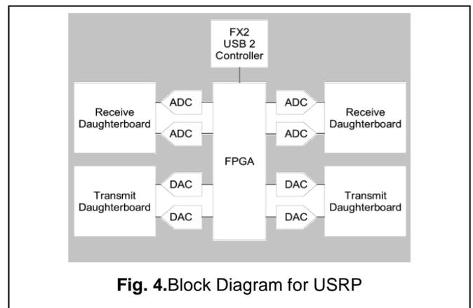
Fig. 4. Block Diagram for USRP
