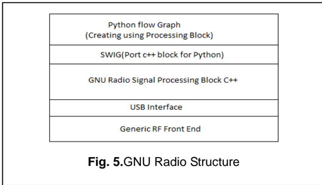
**Fig. 5.** GNU Radio Structure
