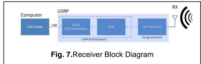
**Fig. 7.** Receiver Block Diagram
