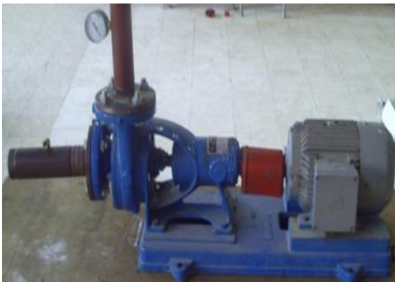
Figure 2.Centrifugal pump of POVAL,type NVA 150-5,[9]
