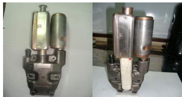
Fig.5.2.1 Existing model Suction head, Modified model Suction head and Suction Valve leaf.
