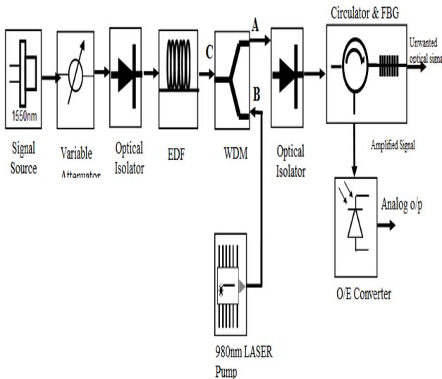
Fig 3: Counter directional pumping
