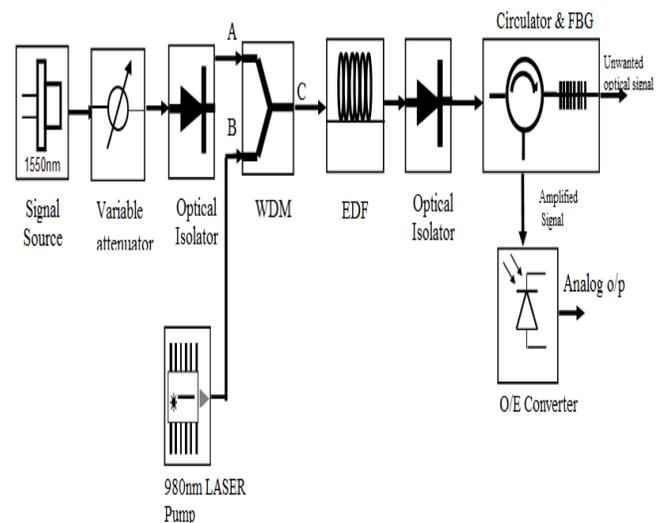
**Fig 2:** Co directional pumping scheme
