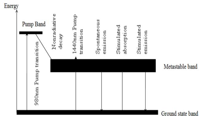
**Fig: 1** Energy level diagram of Erbium ion (Source: Optical Fiber Communication Gerd Keiser)
