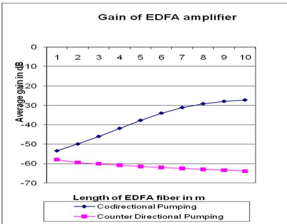
From the above experiments that have been simulated using GainMaster simulation tool we can come to conclusion that the gain of amplifier increases as length of
