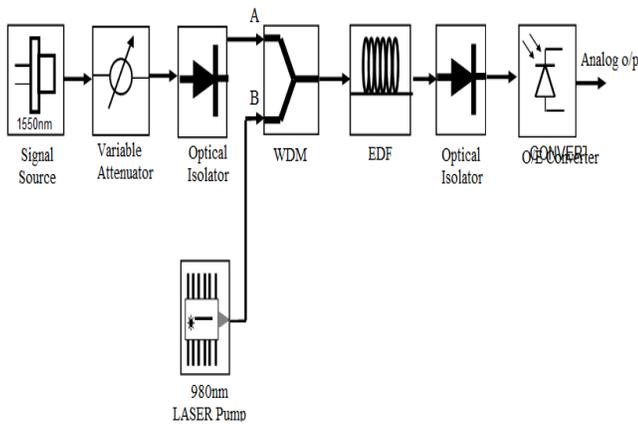
**Fig 5:** Noise Figure measurement
