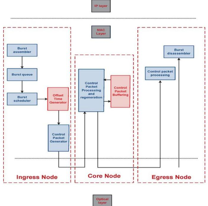
Fig. 3. OBS MAC layer with the proposed CP buffering feature.
