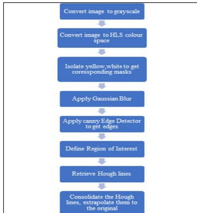
**Fig.2.** Block diagram of Lane detection process.
