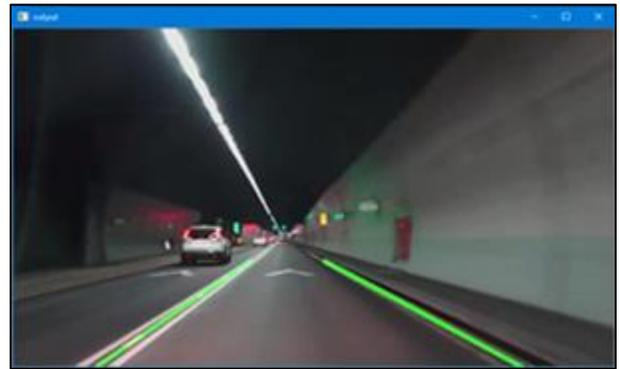
**Fig.3.5** Final Lane line detected output.
