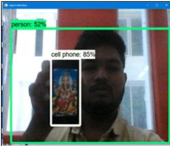
**Fig.3.2** person and cell phone are detected.
