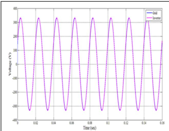
Fig.9. Synchronized between the inverter voltage and the grid voltage.
