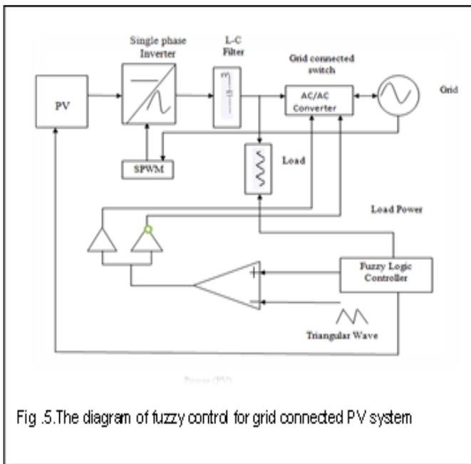
Fig .5. The diagram of fuzzy control for grid connected PV system
