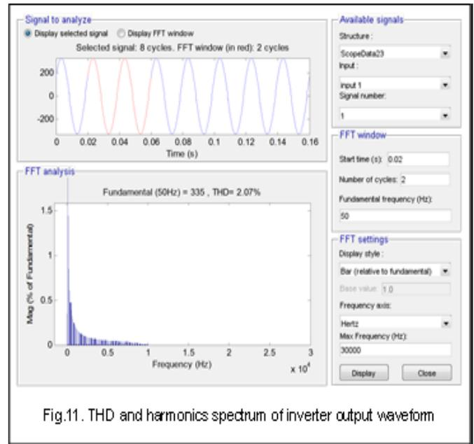
Fig.11. THD and harmonics spectrum of inverter output waveform
