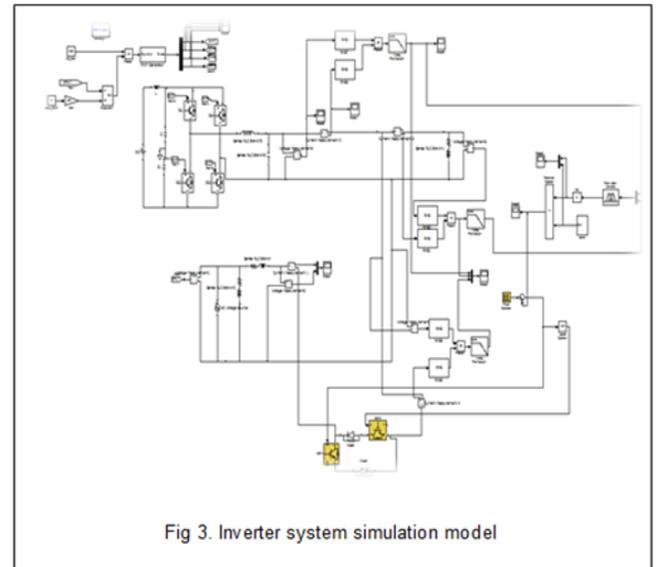
Fig 3. Inverter system simulation model
