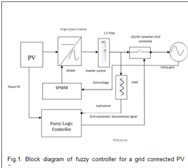
Fig.1. Block diagram of fuzzy controller for a grid connected PV
