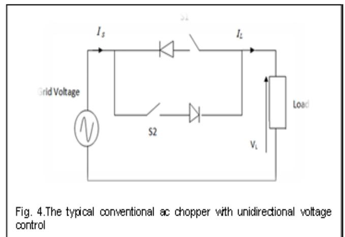
Fig. 4. The typical conventional ac chopper with unidirectional voltage control
