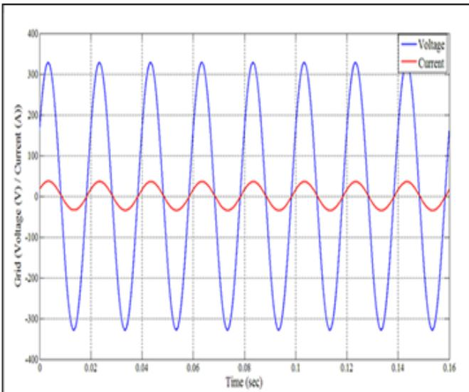
Fig.10. Simulation result Grid voltage and Grid current at unity power
