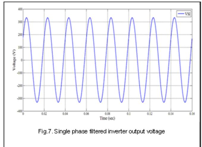
Fig.7. Single phase filtered inverter output voltage
