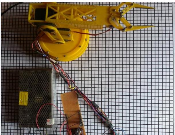
**Figure 7;** testing the robot arm at home position (all servo angles are 90° applied)
