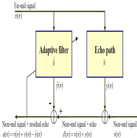
Figure 3. The basic model of Adaptive Filter
