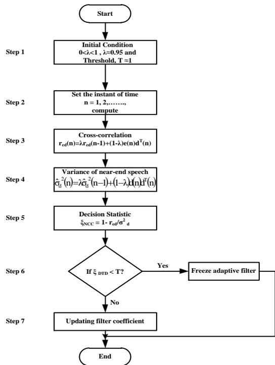
**Step 1:** Initialize condition for this simulation, Threshold,  $T \approx 1$  and  $\lambda = 0.95$ ,  $0 < \lambda < 1$
