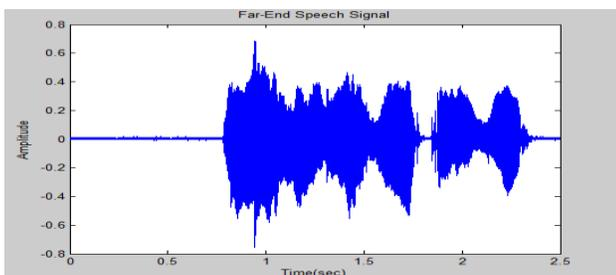
Figure 9. Far-end Speech Signal for LMS and NLMS
