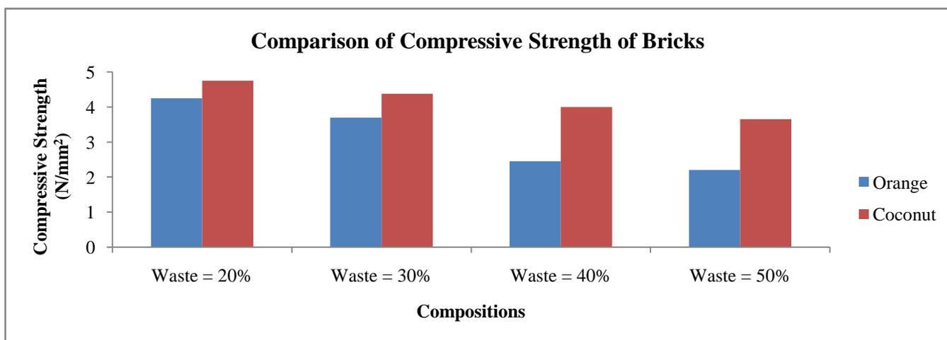
**Fig. No. 4:-** Comparison of compressive strength of bricks when it is prepared by Orange peels and coconut waste.
