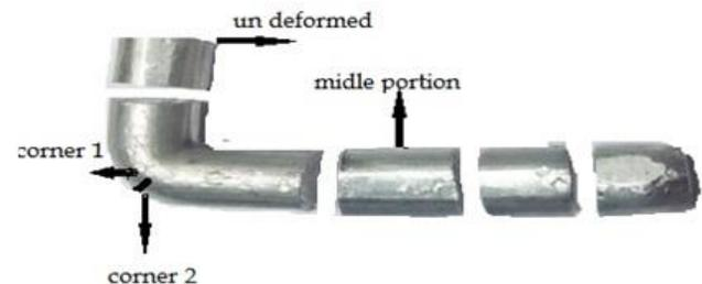
Figure 2: AA 6061 Specimen after ECAP
