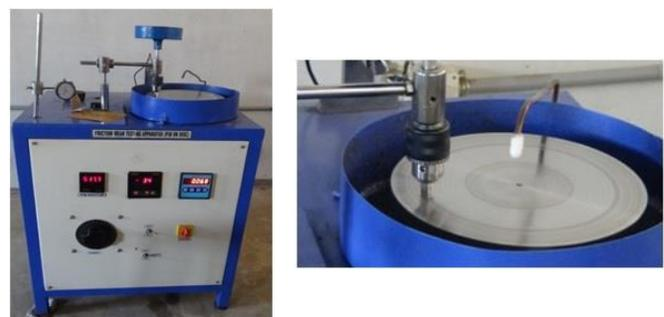
Figure 3: Arrangement of Pin-on-Disk Apparatus
