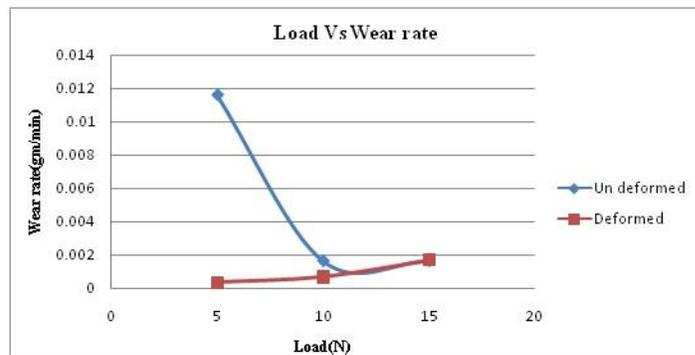
Figure 7: Comparison of Load Vs Wear rate for un-dformed and deformed specimens
