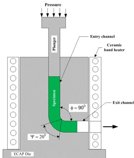
Figure 1: Schematics of equal channel angular pressing
