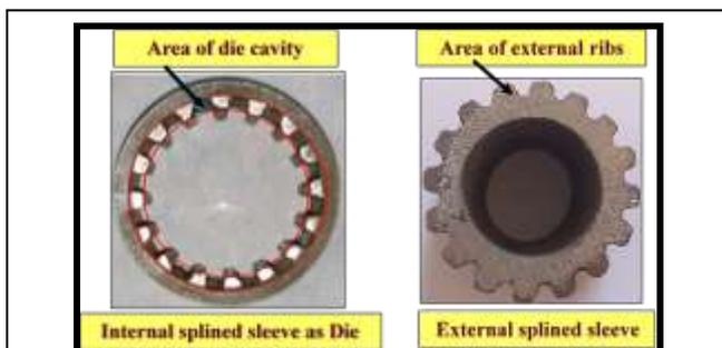
FIG. 6. Photo scan for die and externally splined sleeve products to computed
