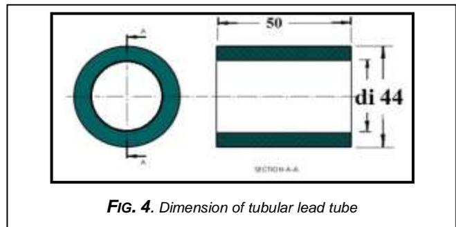
Fig. 4. Dimension of tubular lead tube
