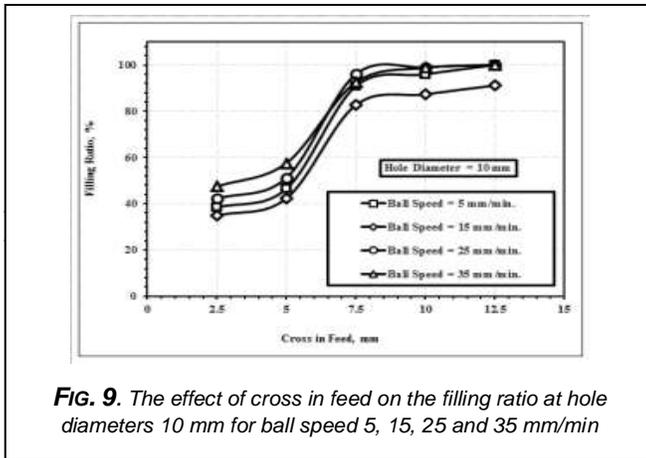
**FIG. 9.** The effect of cross in feed on the filling ratio at hole diameters 10 mm for ball speed 5, 15, 25 and 35 mm/min
