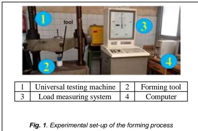
Fig. 1. Experimental set-up of the forming process
