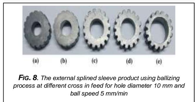
FIG. 8. The external splined sleeve product using ballizing process at different cross in feed for hole diameter 10 mm and ball speed 5 mm/min
