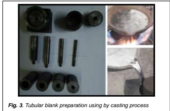
Fig. 3. Tubular blank preparation using by casting process
