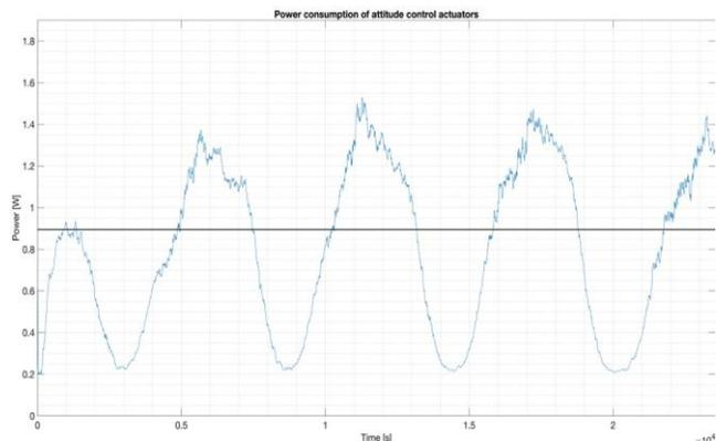
**Fig. 8.** Power consumption of the actuators when the CoM is located in this position:  $CoM = [3.5 \ 3.5 \ 3.5] \text{ cm}$ . ACS turns-on the actuators to produce a corrective torque, with an average of 0.89 W, during the 4 orbit simulation.
