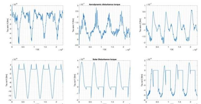
**Fig. 7.** Aerodynamic and Solar disturbance torques actuating on the satellite for four orbits, when the CoM is located on: CoM = [3.5 3.5 3.5] cm.
