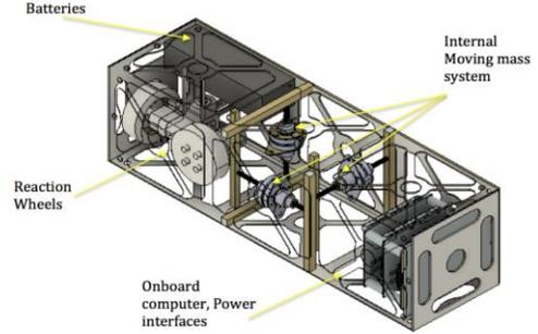
**Fig. 4.** Proposed Internal moving mass system inside a 3U Cubesat structure, showing the three linear motors, the reaction wheels, the onboard computer, and the batteries.
