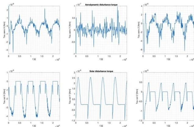
**Fig. 10.** Aerodynamic and Solar disturbance torques on the satellite,  $CoM = [3.0 \ 3.0 \ 3.0] \text{ cm}$ . In this case, disturbance torques has approximately an order of magnitude less than the previous case.
