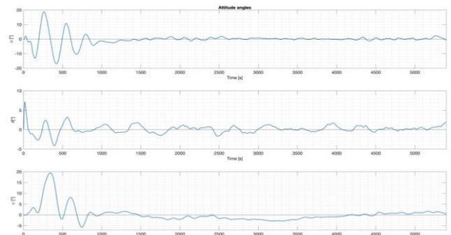
**Fig. 6.** Satellite attitude with CoM = [3.5 3.5 -3.5] cm. The simulation shows large oscillations in the attitude angles due to the disturbance torques, requiring that the attitude subsystem apply stabilization torques.
