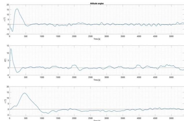
**Fig. 9.** Satellite attitude,  $CoM = [3.0 \ 3.0 \ 3.0] \text{ cm}$ . In this case the attitude is more stable, as the disturbance torques has smaller magnitude.
