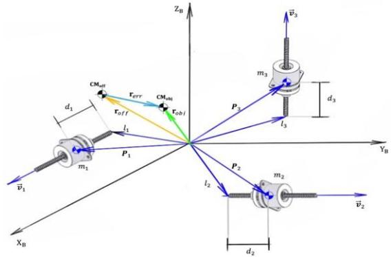
**Fig. 5.** Internal shifting masses system scheme: the displacements of every mass can be denoted by  $d_1, d_2$  and  $d_3$ , respectively, referred to their initial positions.
