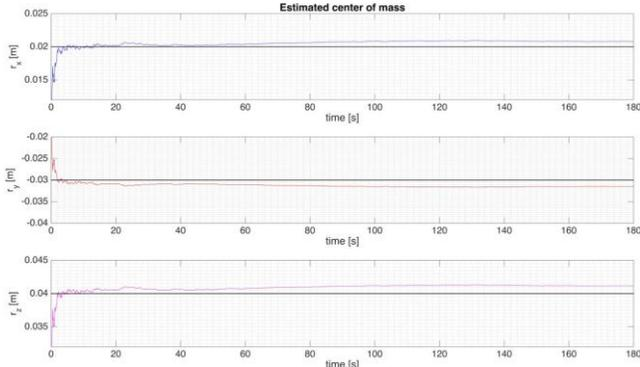
**Fig. 2.** Estimated values of the Center of mass: the simulation shows that the solution converges in approximately 120 s, when these estimated values are stabilized.
