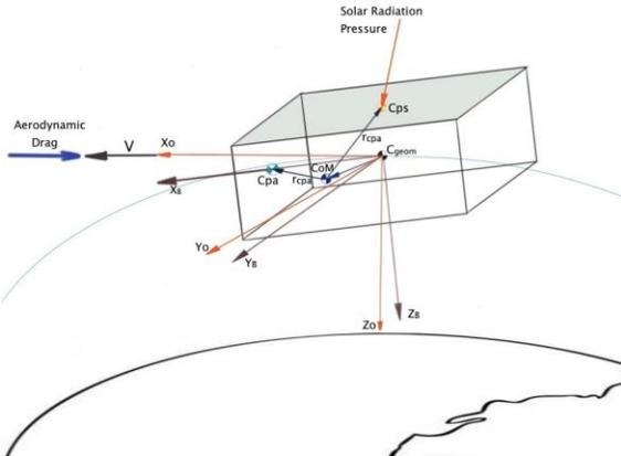
Fig. 1. Coordinate systems for the CoM estimation: Orbital Frame  $X_oY_oZ_o$ , with its origin in the CoM of the satellite,  $X_o$  is tangent to velocity vector  $V$ ,  $Z_o$  points towards Earth's center, and  $Y_o$  completed the orthogonal system. The Body frame  $X_bY_bZ_b$  is a frame aligned with the principal axis of the satellite and moves with it, and it is expected that these two frames be aligned when the desired attitude is reached.
