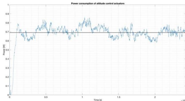
**Fig. 11.** Power consumption of the actuators,  $CoM = [3.0 \ 3.0 \ 3.0] \text{ cm}$ . In this graph is shown that attitude actuators require less power to maintain the attitude, an average of 0.68 [W], and with less oscillations.
