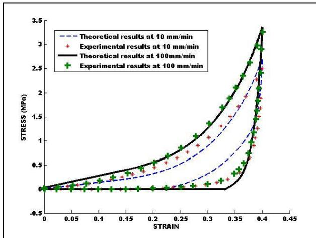
**Figure 7:** Comparison of the experimental data points and the theoretical description computed with Table 1 model constants for the hysteresis loop at 10 and 100 mm/min
