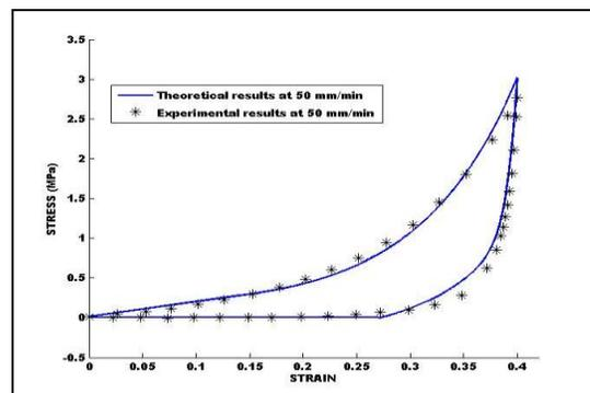
Figure 6: Comparison of the experimental data points and the theoretical description for the hysteresis loop at 50 mm/min
