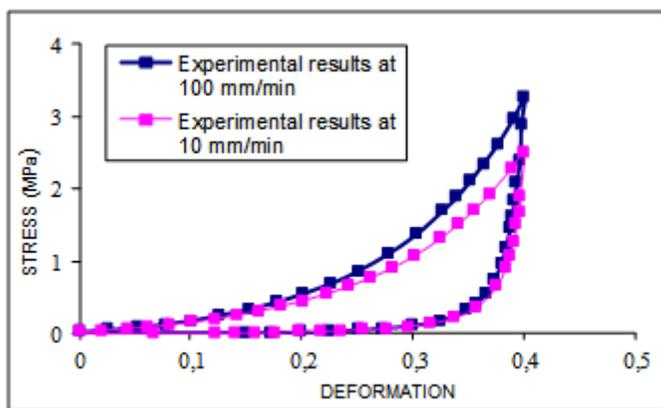
Figure 4: Stress-strain behavior of the knit samples at different strain rates (10 and 100 mm/min)
