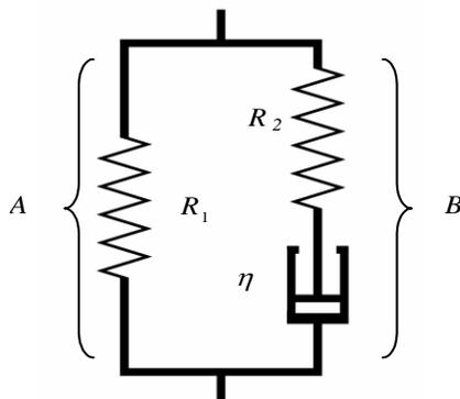
Figure 2: Schematic representation of the Zener viscoelastic model
