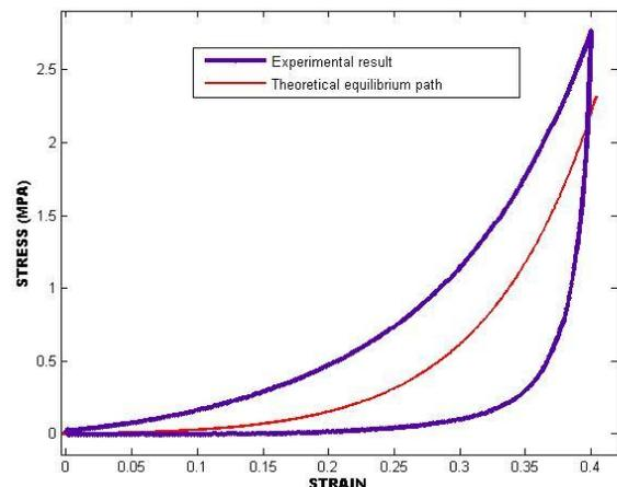
Figure 3: Location of the theoretical equilibrium path relatively to the loading and unloading curves
